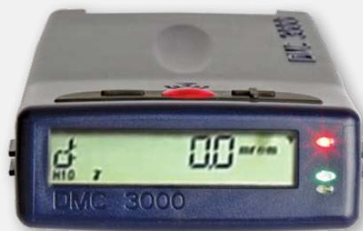
**DMC 3000** family of dosimeters with optional beta, neutron or gamma sensitive PRD modules
