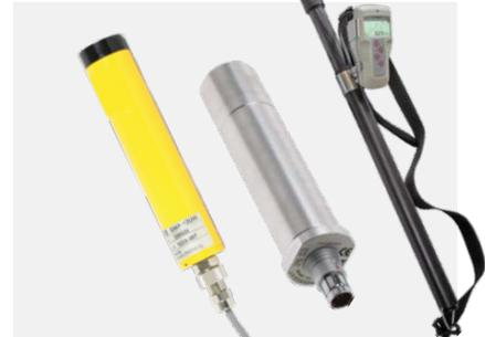
**External and Tele-STC** dose rate probes for high range levels
