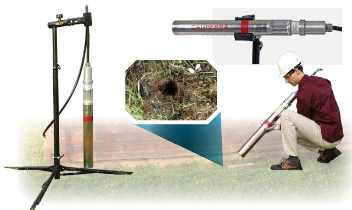
In core spectrometry for Bq/g determination using single sealed LN<sub>2</sub>-free HPGe
