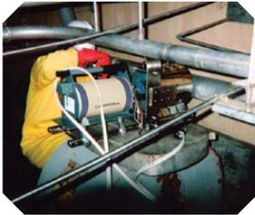
During the dismantling process, materials and other objects will require radioactive quantification. Radiological mapping might also be required in certain areas during the demolition process. Mirion can provide radiological tools and procedures that enable efficient sorting and characterization of waste prior to shipment.
