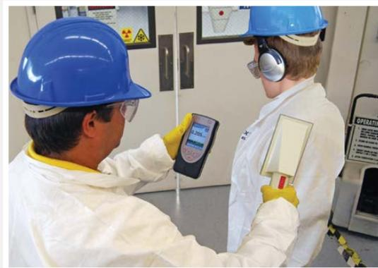
The **Radiagem** and **Colibri** family can accommodate a family of **CSP-Smart probes** for enhanced detection of gamma dose rate and  $\alpha$ - $\beta$  ( $\gamma$ ) contamination monitoring
