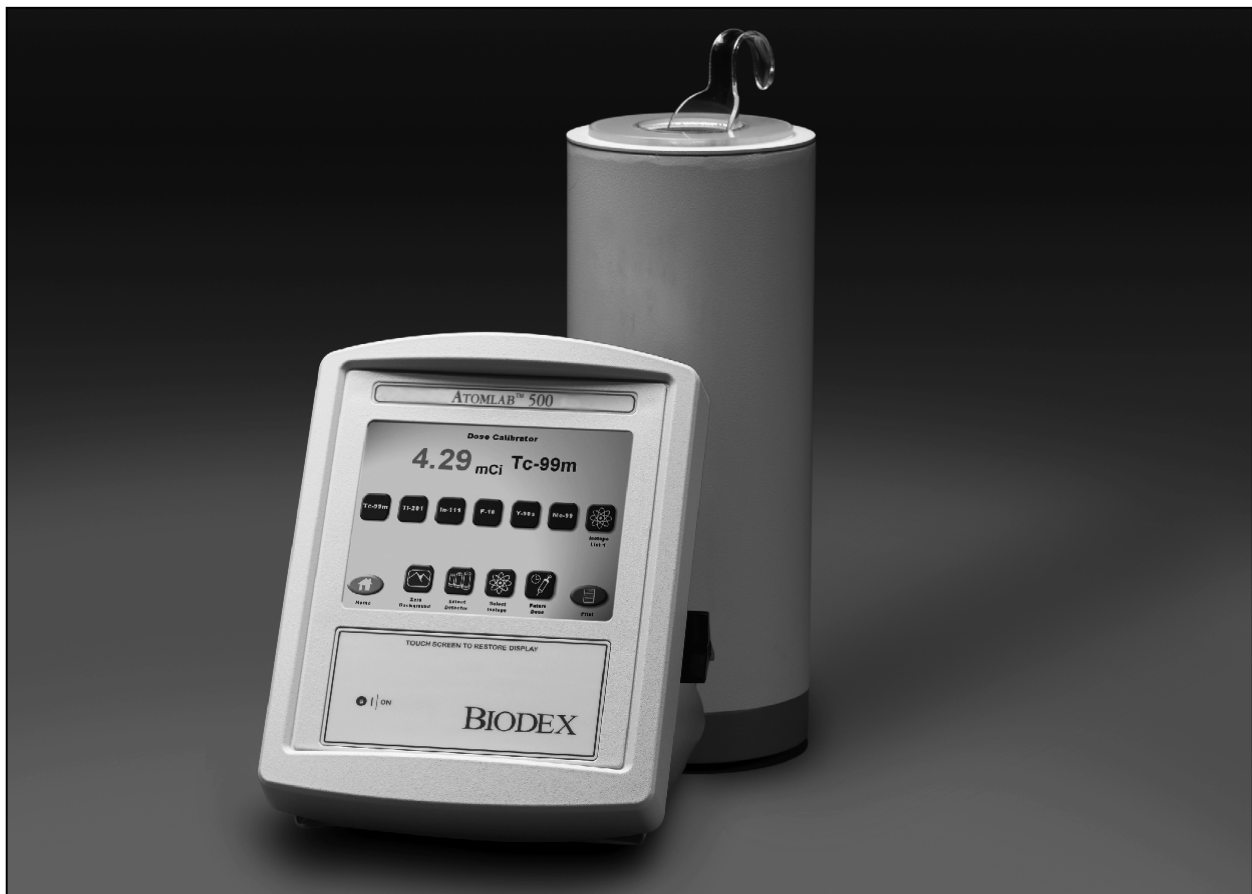
Figure 1.1. The Atomlab 500 features large, easy to read icons, prompts and values on a touch-screen display.
