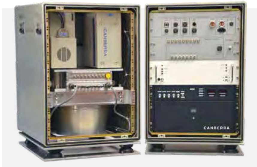
Hardware overview of the Mirion airborne system consisting of two cabinets (detector and processing electronics)
