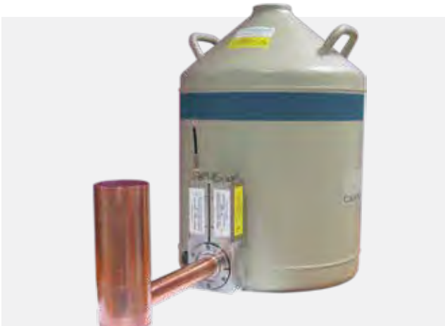
PCGe detector with readout preamplifiers on both detector contacts
