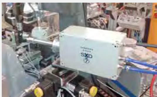
FWHM at 5.9 keV, 7-element detector, each segment 50 mm 2
