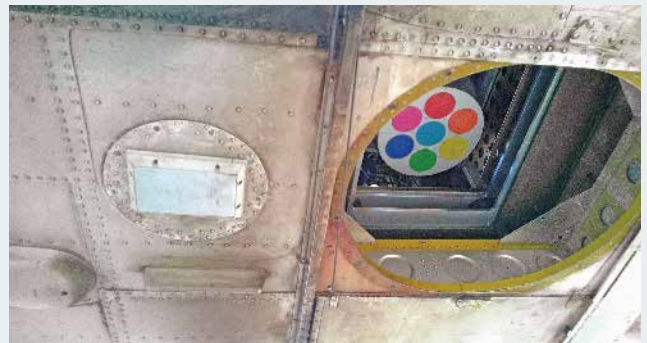
View of detector cap through a hole in aircraft cabin. Each colored circle shows the location of an individual coaxial detector. The seven detectors are in a single common cryostat
