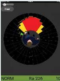
The Radar screen provides direction to the source.
