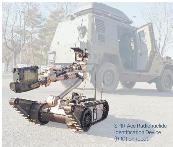
SPIR-Ace Radionuclide Identification Device (RIID) on robot
