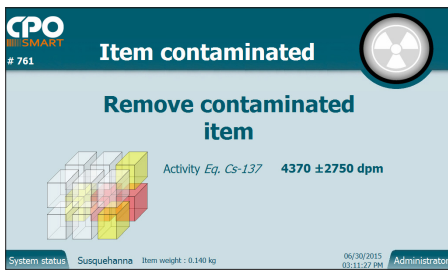
A typical contamination alarm screen
