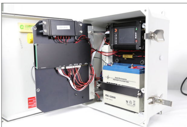
The RBM is completely self-contained in a NEMA certified case, with its own solar power system.
