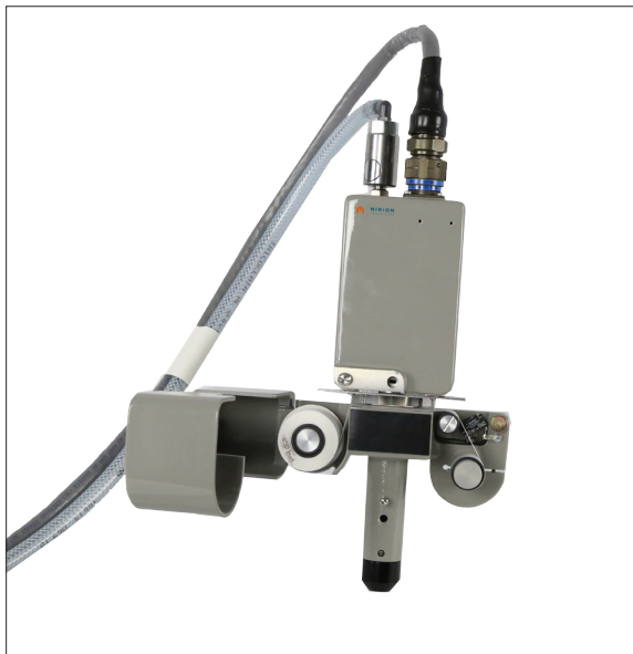
Automatic moving filter head can be located up to 30 ft away
