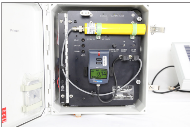
The detection panel can accommodate the RDS-31's various extension probes to meet a variety of measurement needs.
