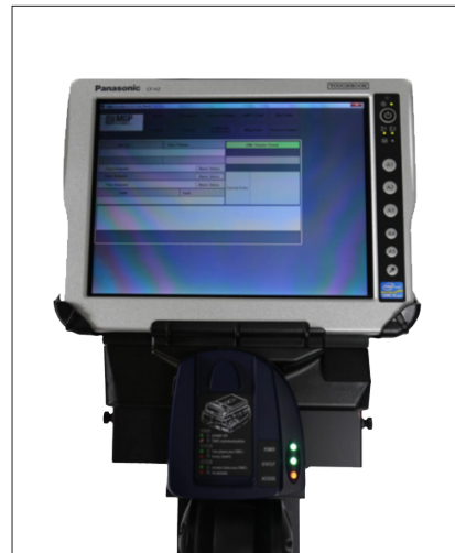
Touch-screen monitor includes 64-bit (Windows 7) OS and TPM Security Chip
