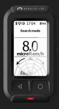
The AccuRad<sup>™</sup> PRD is a Personal Radiation Detector (PRD) designed for law enforcement, fire and rescue, and other emergency responders to detect and interdict nuclear and radioactive materials. It also provides dose measurement and alarming capabilities for event response.
