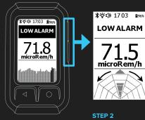
STEP 1 Press either arrow on side of device to enable Search mode AccuRad PRD assists with locating the source (See next page)
