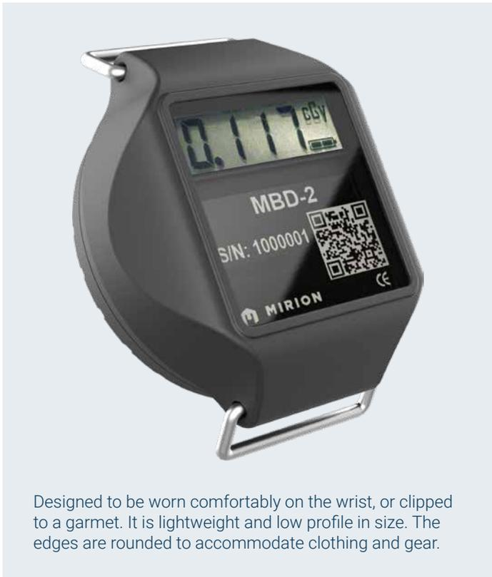
Designed to be worn comfortably on the wrist, or clipped to a garmet. It is lightweight and low profile in size. The edges are rounded to accommodate clothing and gear.
