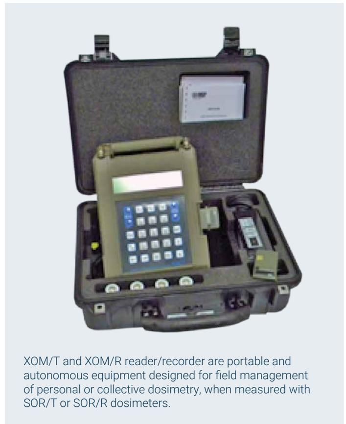
XOM/T and XOM/R reader/recorder are portable and autonomous equipment designed for field management of personal or collective dosimetry, when measured with SOR/T or SOR/R dosimeters.
