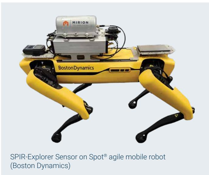
SPIR-Explorer Sensor on Spot® agile mobile robot (Boston Dynamics)
