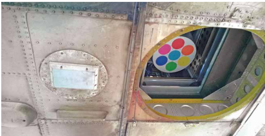
View of detector cap through a hole in aircraft cabin. Each colored circle shows the location of an individual coaxial detector. The 7 detectors are in a single common cryostat.
