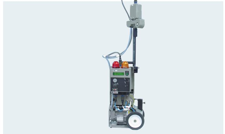
ABPM 203M™ Mobile Alpha/Beta Particulate Monitor. This monitor, with its small and lightweight extendable sensor, functions locally next to the respiratory tract of workers. It is perfectly adapted for the measurement of particulates in environments with high rates of radon.
