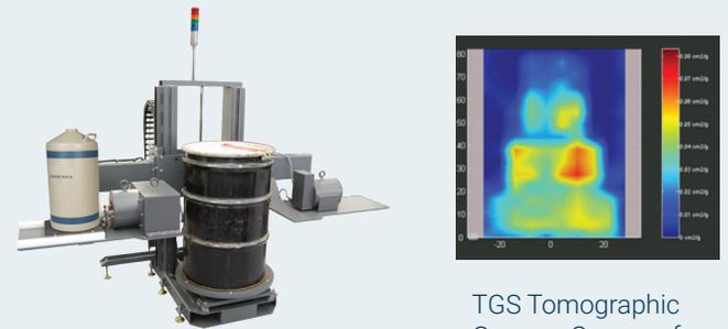
SGS Segmented Gamma Scanner for Waste Characterization
