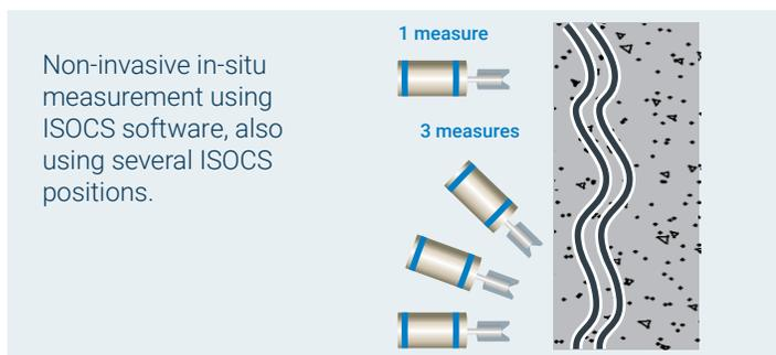
Wall or surface determination in Bq/cm<sup>2</sup> and in-depth profile detection using ISOCS HPGe
