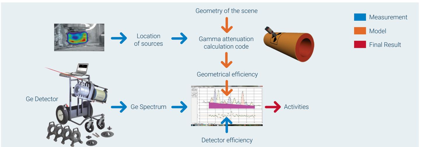
ISOCS Uncertainties Estimator and multi-Geometry Calculator enables the testing of the sensitivity of model's parameters, such as geometry, material, shapes, etc.
