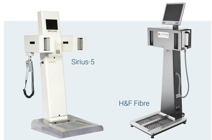
Sirius™-5 (gas or gasless) and H&F Fibre (gasless) for  $\alpha$ - $\beta$  contamination monitoring purposes
