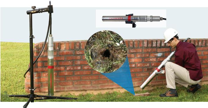
In-core spectrometry for Bq/g determination using single sealed LN<sub>2</sub>-free HPGe
