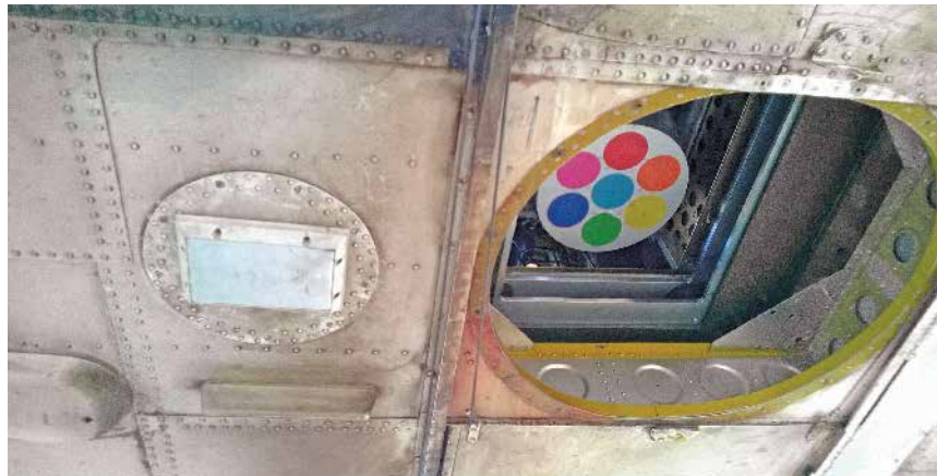
View of detector cap through a hole in aircraft cabin. Each colored circle shows the location of an individual coaxial detector. The 7 detectors are in a single common cryostat.
