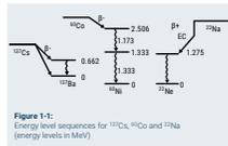
Figure 1-1: Energy level sequences for <sup>22</sup>Na, <sup>60</sup>Co and <sup>137</sup>Cs (energy levels in MeV)
