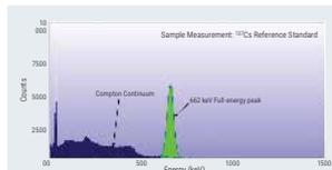
Figure 1-3: Example spectrum of a <sup>137</sup>Cs source
