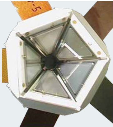
Si(Li) array for backscattered X-ray detection
