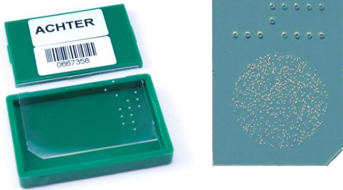
Figure 3: Left: opened PADC-dosimeter showing foil. Right: example of an etched foil.
