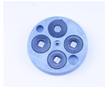
Figure 2: The TL- dosimeter seen from the inside: above the beta detector, to the left and right the photon detectors and below the neutron detector.
