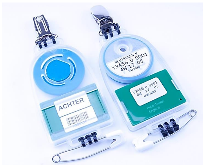
Figure 1: The combi-dosimeter consisting of the combination of a TL-dosimeter (above) and a PADC-dosimeter.
