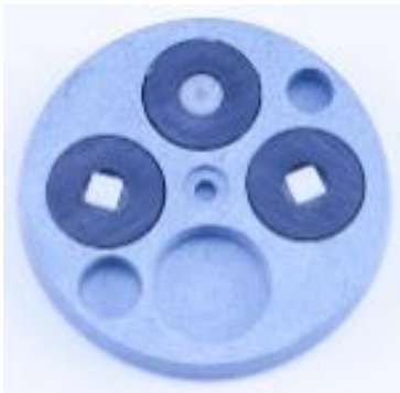
Figure 1: The grey beta/photon dosimeter seen from the inside: above the beta detector and to the left and right the photon detectors, as they are also present in the (green) photon dosimeter.
