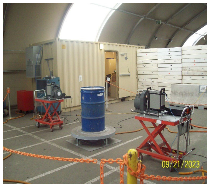
Figure 1. MILCC1 at LANL, two AEGIS™ detectors on carts, with rotator in the middle.
