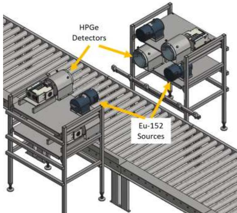
Figure 1 BMS detectors (4) and Transmission sources (4)
