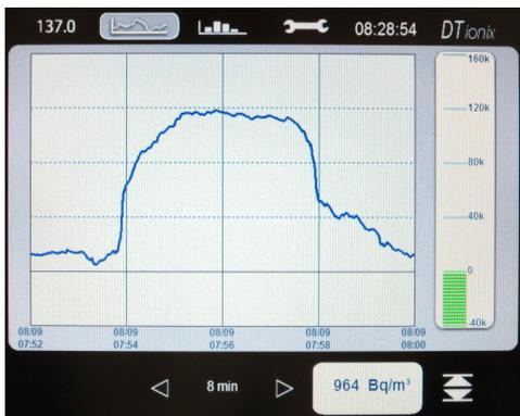
Injection of 100 kBq/m<sup>3</sup> (2.7 μCi/m<sup>3</sup>) in a C IONIX 3 - BMM
