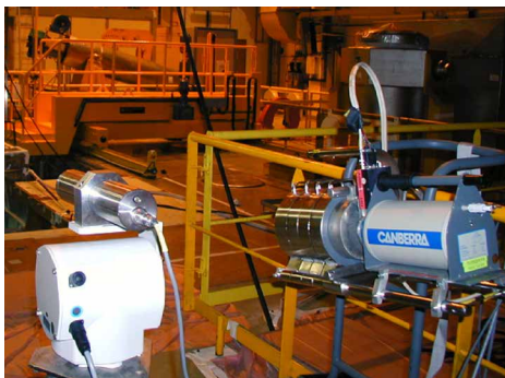
Figure 6. At the left the CAROGAM unit finds sources, at the right the ISOCS software qualitatively and quantitatively measures radioactive isotopes
