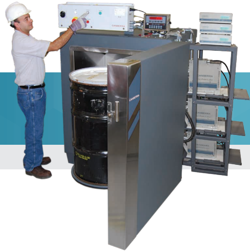
Figure 1: The Model WM2110 Germanium Q 2 Low Level Waste Assay System.
