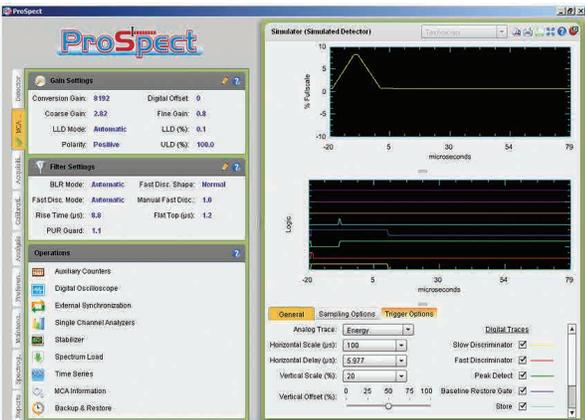
For the Lynx unit, access to a Digital Oscilloscope is provided. When invoked, this occupies the main panel of the screen to allow a concurrent view of the MCA setting editing and the analogue and digital traces facilitating the set-up of MCA hardware.
