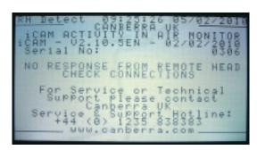
Normal operation is restored automatically once communications are restored.
