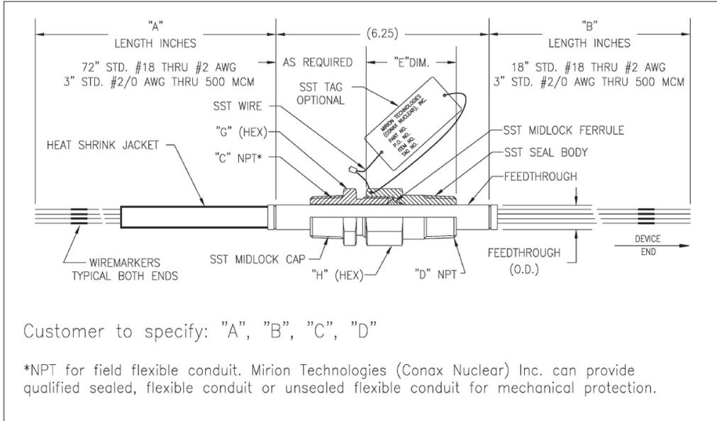
Diagram of Electric Conductor Seal Assembly (ECSA)
