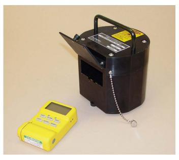
\* If calibration check falls outside the tolerances, UltraRadiac needs to be re-calibrated in CANBERRA™ Services with NIST traceable calibrator.
