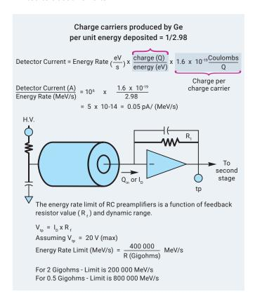
The energy rate limit can be increased very substantially by choosing a lower value feedback resistor with, of course, an accompanying increase in noise. Actual performance data on a typical detector is given in the following table:
