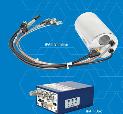
Optimized to perform high-resolution gamma spectroscopy and timing measurements, the iPA II is a low-noise, high speed resistive feedback preamplifier for High Purity Germanium (HPGe) detectors, enabling extensive control and monitoring of critical State-of-Health parameters of the preamplifier and detector.
