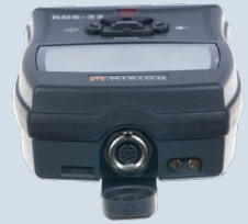
Connector, charging contacts, fixing lug for wrist strap
