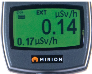
Display with Gamma Probe
