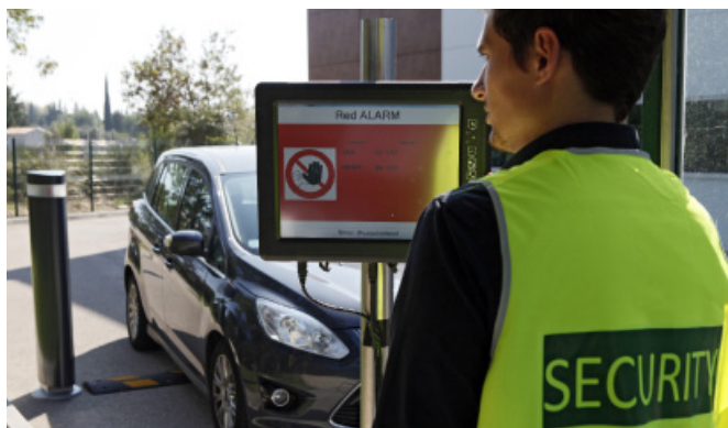
Double-sided SPIR-Ident Pedestrian monitor with green/red alert screen.
