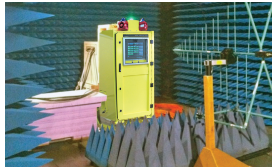
EMC Tests on the CAAS Cabinets
