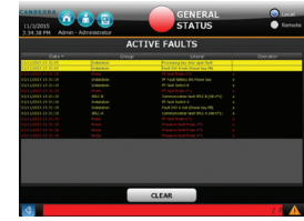
Red for major fault: the safety function is potentially affected (alarms might not be issued in case of criticality accident)
