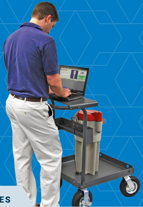
**A complete, transportable food analyzer for quickly determining whether raw or processed food has become contaminated from a radiological event.**
