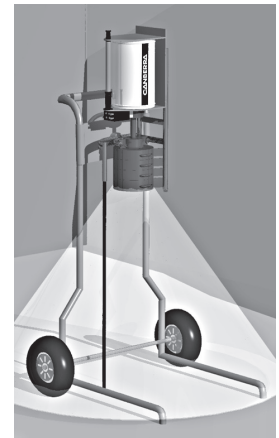
7b: Shield and collimator installed.
