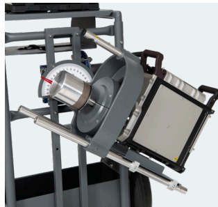
5a: The detector and mounting assembly. The red indicator enables an accurate reading of the detector tilt angle. Note that the detector has the RDC chamber and that the backshield is installed.
